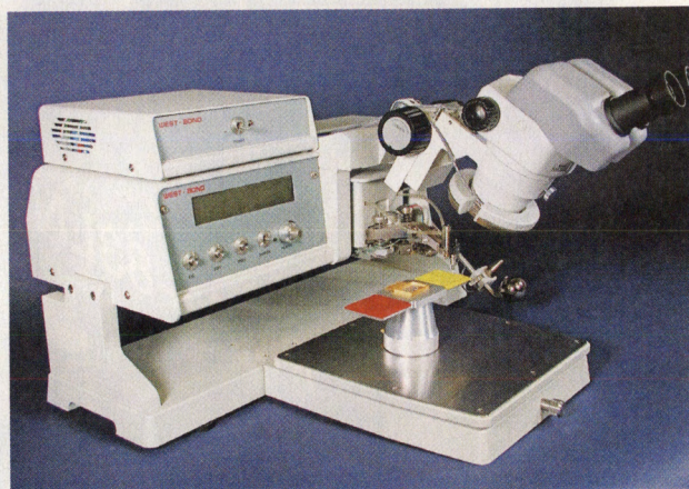
1. Both epoxy and eutectic bonding are handled by this die bonder. (Courtesy of West-Bond)
